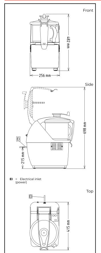
Electric Supply voltage: 200-240 V/1N ph/50/60 Hz Electrical power, max: 1.3 kW **Total Watts:** 1.3 kW Capacity: Performance (up to): 2.5 kg/Cycle **Capacity:** 5.5 litres Key Information: External dimensions, Width: 256 mm External dimensions, 415 mm Depth: External dimensions, Height: 482 mm **Shipping weight:** 23 kg
